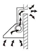
3.1 The cooker hood should be placed at a distance of 65-75cm above the cooking surface for the best effect.
